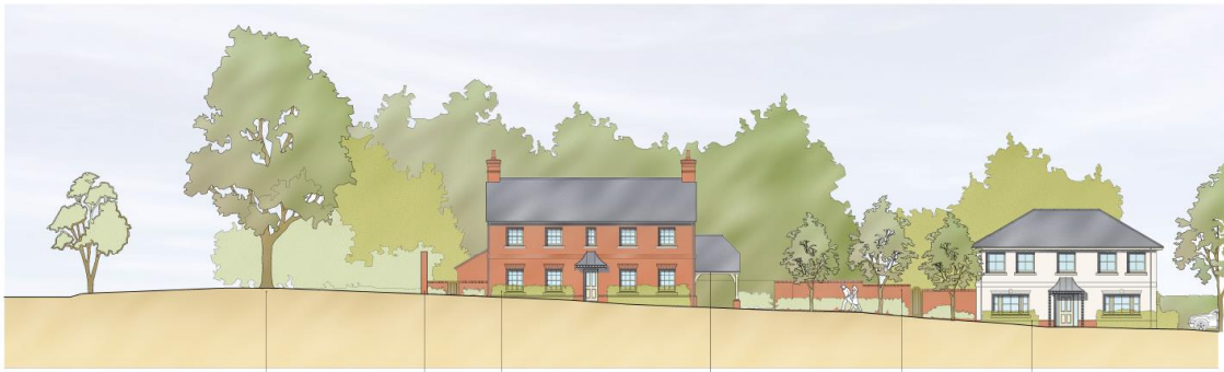
Harvest Hill Road Section AA (Front) 1:100 TPO Oak Existing wall and opening retained Low level railings Plot 1 Front elevation Garport Plot 1 Proposed garden wall Low level railings Plot 2 Front elevation
